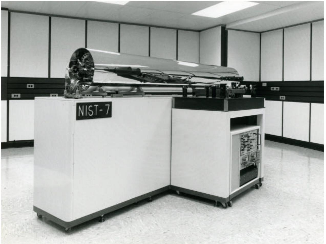
NIST-7 is the cesium-beam primary frequency standard for the United States. At an accuracy of  $1 \times 10^{-14}$ , this standard contributes significantly to the accuracy of the rate of international time and lends long-term stability to NIST's time scale. The standard also serves as a reference in evaluating the performance of advanced commercial frequency standards. (*Courtesy of NIST, the National Institute of Standards and Technology*)
